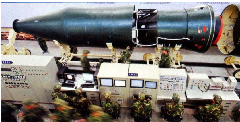
The February 2009 issue of PLA Pictorial included this image of the third stage of the DF-31A ICBM. It shows multiple thrusters on the base of the stage and the shroud suggests there is space for multiple warheads, or for one warhead and multiple decoys.
