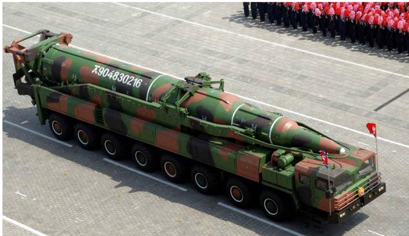
**Solid or Liquid:** A solid fueled missile of this size would represent a major North Korean advance in missile capability, one that likely has been a result of China's direct sale or transfer of technology, as with the missile's TEL.
